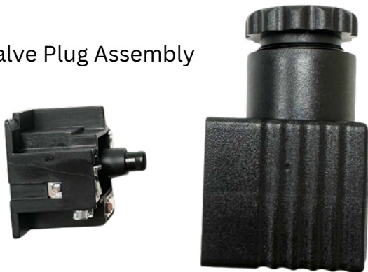
Terminal 1 = Brown Terminal 2 = Blue Centre Earth - NOT USED
