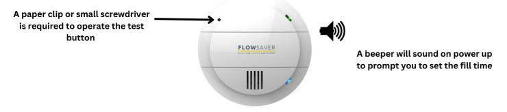
3. To set fill time press and hold the TEST button for 3 seconds until both LEDs are off. The valve will now be open and water will flow into the cistern. During filling the green LED will flash once every 2 seconds. When the cistern has filled with water and flushed the TEST button should be pressed again to record the fill time. This cistern fill time value will be stored in the system memory. The fill time can't be less than 1 minute, if it is slow the water down via an isolation valve.
