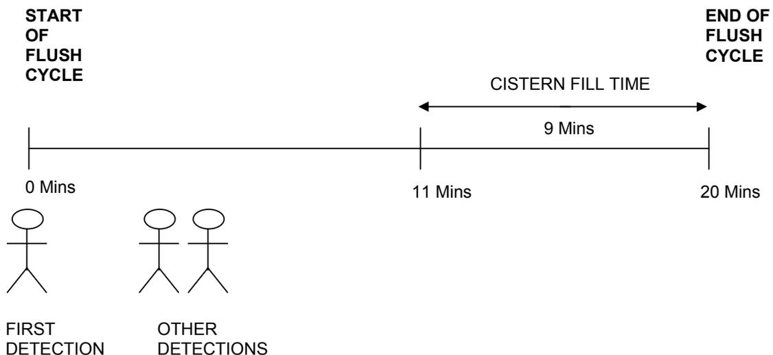
The cistern fill time is the time for which the valve is open during a flush cycle and is set once by the installation engineer. This fill time will vary from one cistern to the other depending on its size and the rate at which the cistern fills. By setting up the fill time for each individual cistern, optimum water savings can be achieved.
